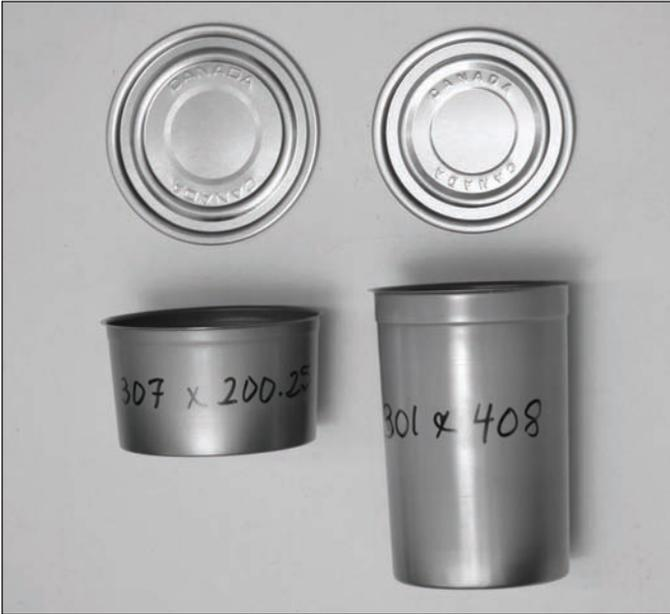
To assemble the sealer, you will need to identify the can size you will be using (diameter and height). The size of the can will determine the:
