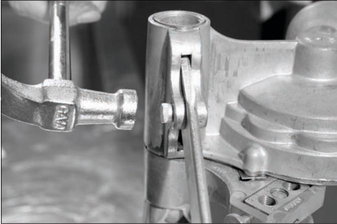
Insert the lever pivot from the back—knurled (ridged) side of the pivot out. Tap in the lever pivot with a hammer.
