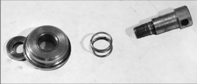
Make the first roller assembly by putting the spring onto the roller screw, then the seaming roller, and then the washer. The largest part of the seaming roller is next to the washer.
