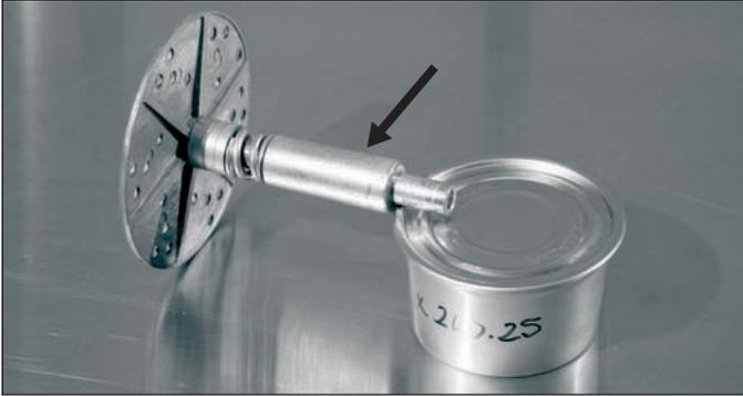
Select the required spacers and extension for your can size (see page 14). Place the spacers, then the spring onto the shaft of the turntable. For the 307 x 200.25, ½-pound flat salmon can, the turntable extension is required (arrow).
