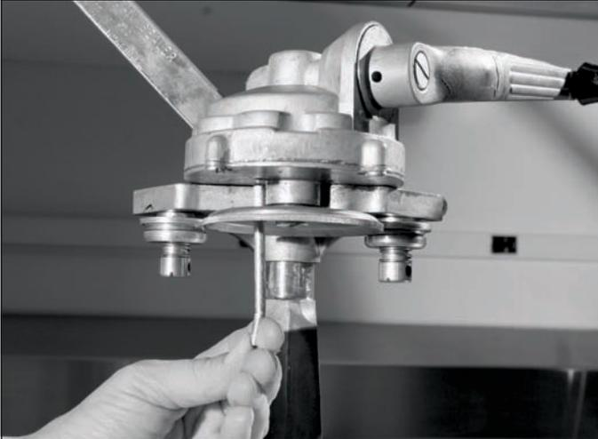
Insert the 3-inch pin into one of the small holes in the chuck. Turn the crank clockwise until the 3-inch pin is pressed against the frame and chuck is tight. Remove the pin.
