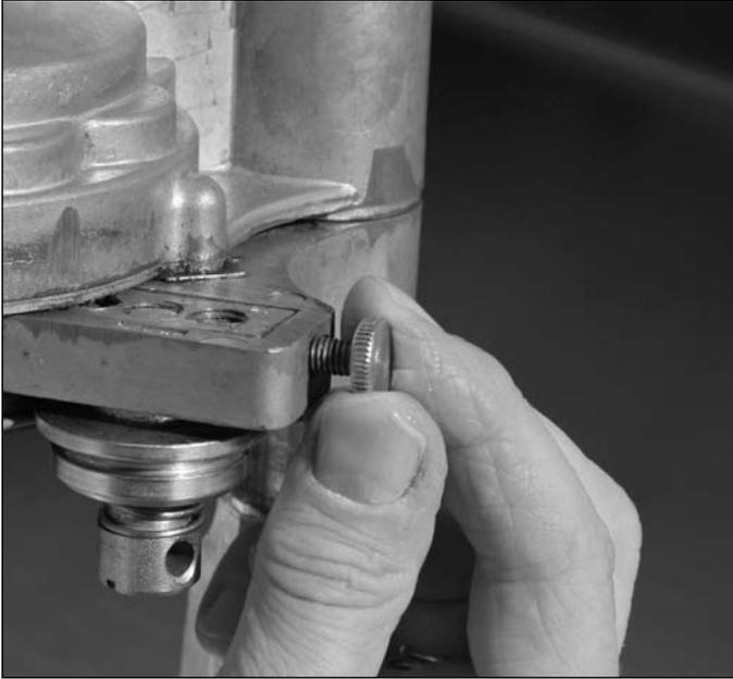
Thread in the thumbscrew loosely. Rotate the crank until the “1” appears in the indicating window.
