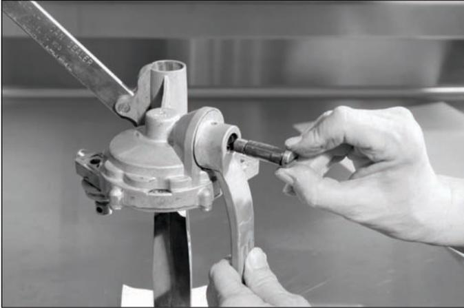
Insert the gear end of the crank into the head. Thread the screw.
