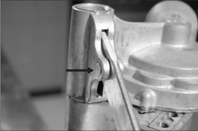
The lever pivot should be flush with the backside of the head (arrow).
