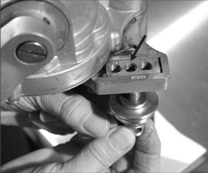
Loosely thread the first seaming roller assembly into the 3-hole nut from the bottom.
